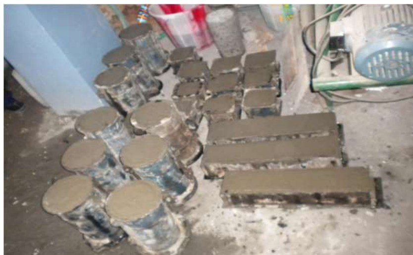
Figure Fresh Concrete Mix in Mould
